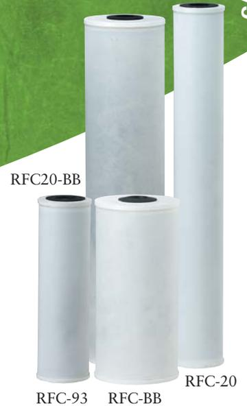
RFC Series cartridges are constructed with a 70-micron porous polyethylene outer shell and durable polypropylene end caps. The 2-3/4" OD cartridges have a polypropylene core and the 4-1/2" OD cartridges incorporate a spun polypropylene core. Sandwiched between the outer shell and the core is a bed of granular activated carbon (GAC).
